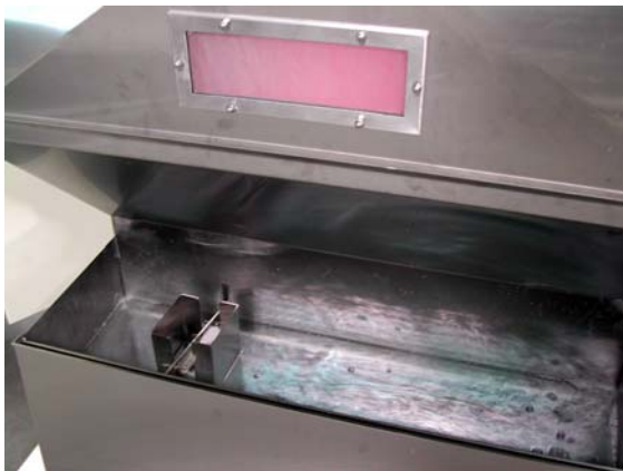
Stainless cover slides back to reveal water tank. Float valve is contained in waveless chamber. Window provides view of spray and flame interaction during operation.
