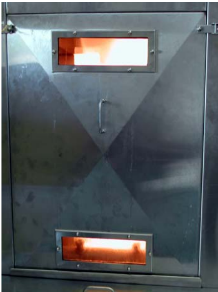
Fire and water combine in this view through the windows of the Sahara at maximum output. More than 4 gal/min evaporation is possible for extreme ginning conditions.
