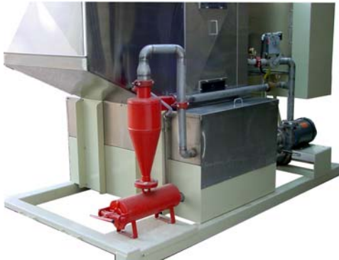
Hydrocyclone filter keeps water tank clean
