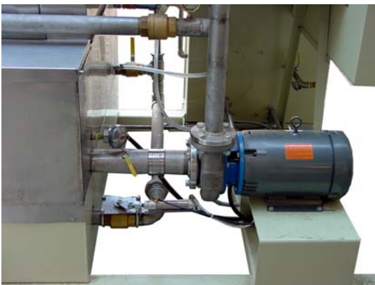
7-1/2 HP cast stainless pump delivers performance
