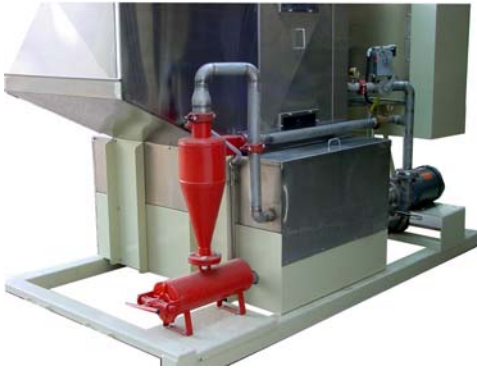
Hydrocyclone filter keeps water tank clean
